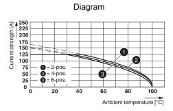
PC 35 HC/..-STF-15,0 with IPC 35 HC/..-STGF-15,0 Derating curve, representation based on DIN EN 60512-5-2:2003-01 Connected conductor cross section = 35 mm<sup>2</sup> Reduction factor = 0.8 Number of positions: see diagram
