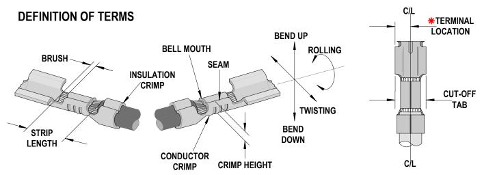
\*Terminal is to be centrally located between the two (2) cut-off tab edges by one half of the total cut-off tab tolerance.
