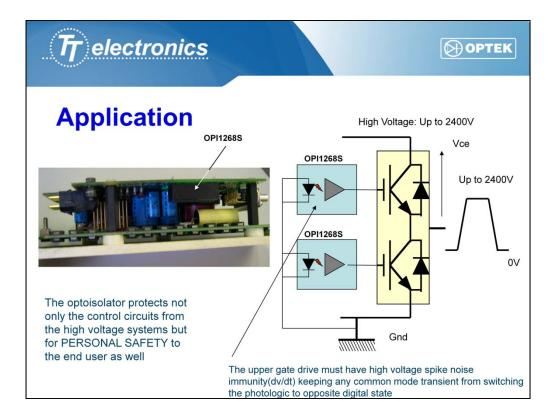
An optoisolator is used in any application that requires isolation between a low voltage control circuit and a high voltage work circuit.
