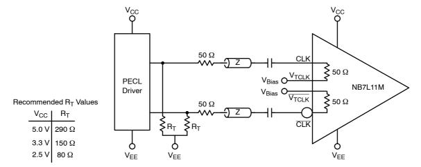
Figure 16. PECL to CML Receiver Interface
