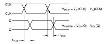
Figure 8. AC Reference Measurement
