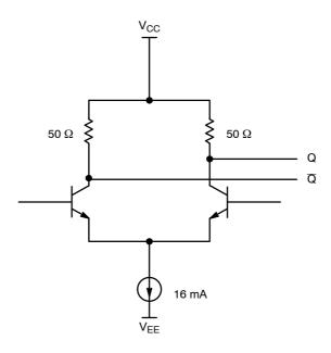
Figure 14. CML Output Structure
