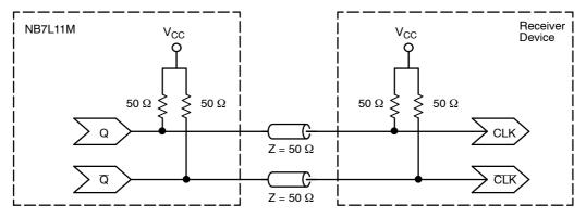
Figure 9. Typical Termination for Output Driver Using External Termination Resistor (Refer to Application Notes AND8020/D and AND8173/D)
