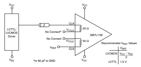
Figure 18. LVCMOS/LVTTL to CML Receiver Interface
