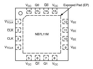
Figure 2. QFN-16 Pinout (Top View)
