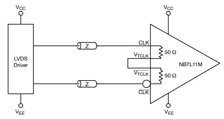
Figure 17. LVDS to CML Receiver Interface
