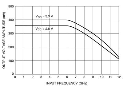
Figure 3. Output Voltage Amplitude ( $V_{OUTPP}$ ) versus Input Clock Frequency ( $f_{in}$ ) at Ambient Temperature (Typical) ( $V_{INPP} = 400 \text{ mV}$ )
