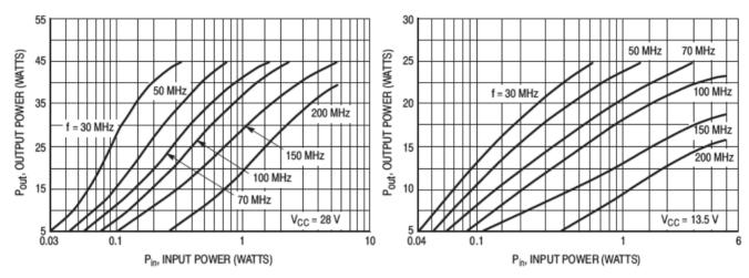
Figure 2. Output Power versus Input Power
