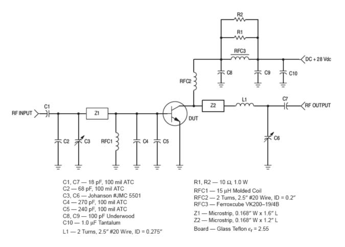
Figure 1. 150 MHz Test Circuit
