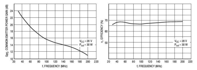
Figure 4. Power Gain versus Frequency
