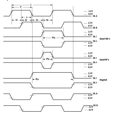
Figure 1. Output waveforms for counter-clockwise rotation, viewed from the top of the encoder.
