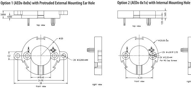
CAUTION: For optimal performance, base plate and plastic housing assembly are designed for a ONE time assembly process only. Removal and re-assembly process should be avoided due to the potential weakness of the latch after re-assembly.
