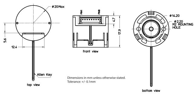
Figure 3. Mechanical Dimensions for Mounting Option 2 (AEDx-8x1x)
