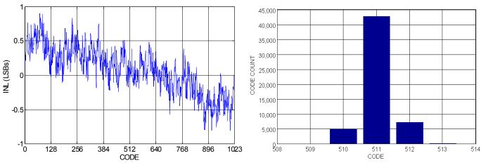
FIGURE 11. INTEGRAL NONLINEARITY vs OUTPUT CODE
