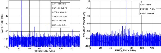
FIGURE 15. OUTPUT SPECTRUM; fIN = 300MHz
