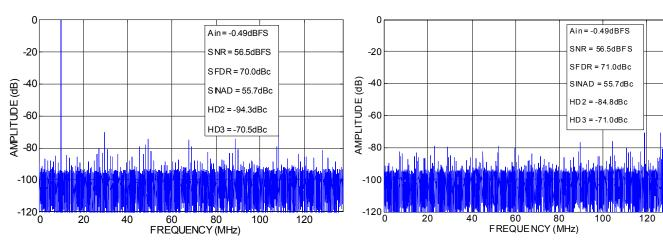
FIGURE 13. OUTPUT SPECTRUM;  $f_{IN} = 10MHz$
