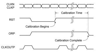
FIGURE 21. CALIBRATION TIMING
