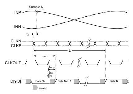
FIGURE 1. LVCMOS TIMING DIAGRAM
