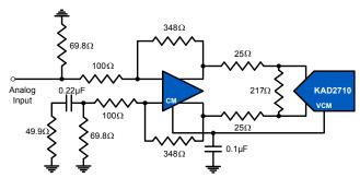
FIGURE 25. DIFFERENTIAL AMPLIFIER INPUT
