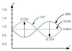
FIGURE 22. ANALOG INPUT RANGE
