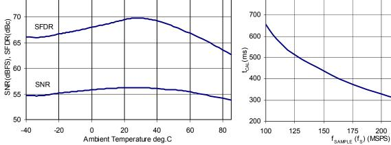
FIGURE 19. SNR vs TEMPERATURE
