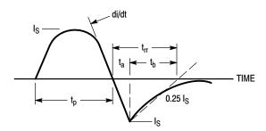
Figure 14. Diode Reverse Recovery Waveform
