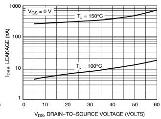
Figure 6. Drain-to-Source Leakage Current versus Voltage
