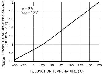
Figure 5. On–Resistance Variation with Temperature
