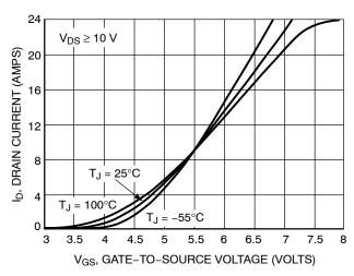
Figure 2. Transfer Characteristics
