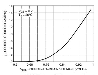
Figure 10. Diode Forward Voltage versus Current
