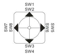
Two switches will actuate in each of the four directions: North, South, East & West.
