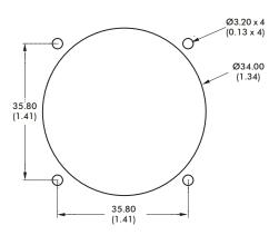
The joystick flange is mounted beneath the panel and the base of the boot must be brought through the panel cut-out and held in place with the circular bezel (option 4). For panel thicknesses of 3mm, M3 x 16 countersunk machine screws are recommended.
