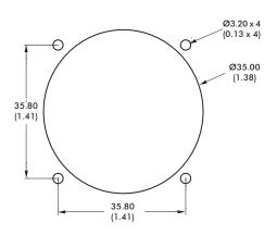
When mounted this way the panel acts as the bezel and no separate bezel is needed. M3 machine screws are recommended.
