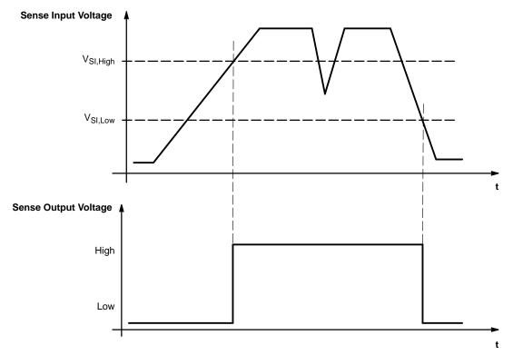
Figure 4. Sense Timing Diagram
