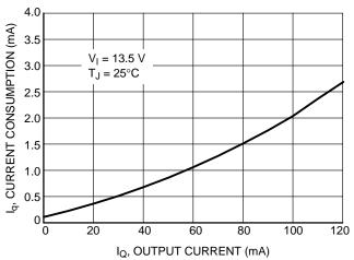
Figure 14. Current Consumption  $I_q$  vs. Output Current  $I_Q$
