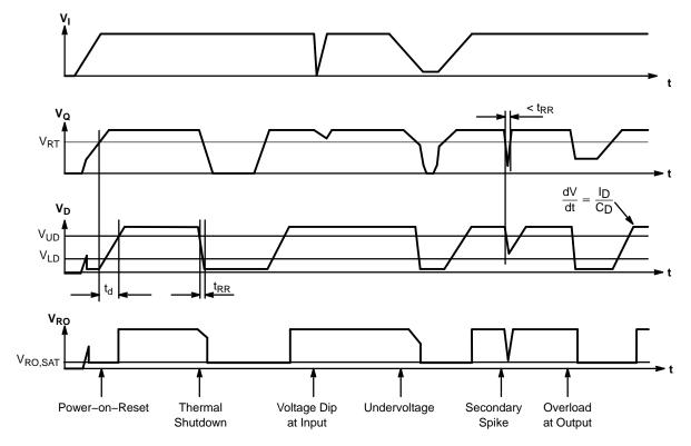
Figure 3. Reset Timing Diagram
