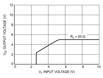
Figure 10. Output Voltage  $V_Q$  vs. Input Voltage  $V_I$
