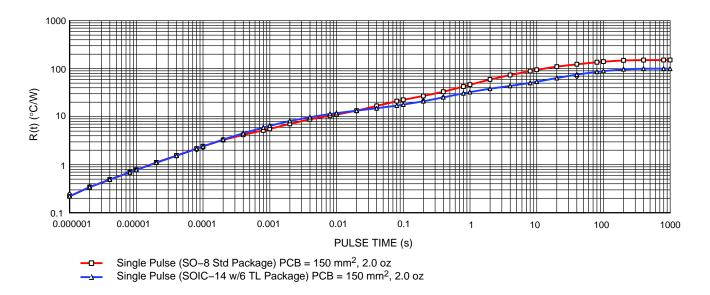
Figure 20. R(t) vs. Pulse Time
