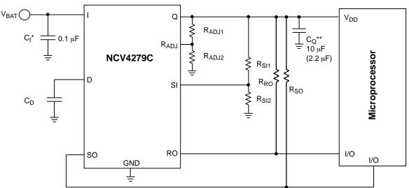
\*C<sub>I</sub> required if regulator is located far from the power supply filter.
