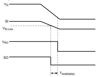
Figure 22. SO Warning Waveform Time Diagram
