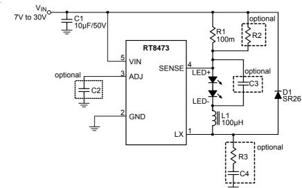
$V_{IN}$  = 7V to 30V  $V_{OUT}$  = 3.5V  $I_{OUT}$  = 1A
