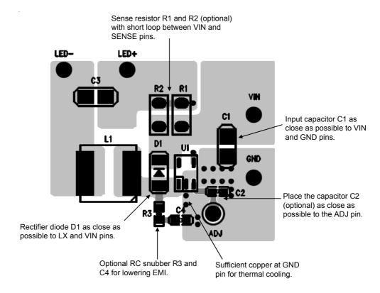
Figure 3. PCB Layout Guide (Top Layer)
