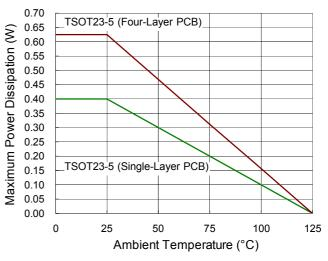
Figure 2. Derating Curves for the RT8473 Packages
