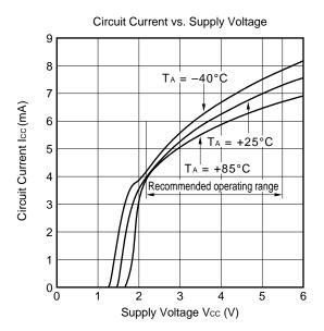
Divide by 2 mode (Guaranteed operating window:  $V_{CC} = 2.2$  to 5.5 V,  $T_A = -40$  to +85°C)
