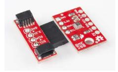
Once you've got headers soldered onto each of your boards, simply plug your adapter into your I<sup>2</sup>C enabled device. Using a Qwiic cable, plug your Qwiic adapter into a stackable Qwiic board of your choice. Assuming that there is example code loaded on your development board, you can now start reading data from your I<sup>2</sup>C enabled device!
