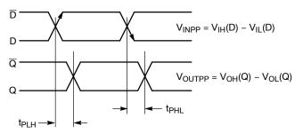
Figure 5. AC Reference Measurement
