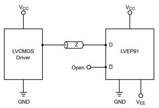
Figure 11. Standard LVCMOS Interface (D will default to  $V_{CC}/2$  when left open. A reference voltage of  $V_{CC}/2$  should be applied to D input, if  $\overline{D}$  is interfaced to CMOS signals.)
