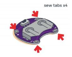
We recommend using a small dot of hot glue (preferred) or fabric glue to attach each LilyPad piece to the fabric to keep it from moving while you sew. Make sure not to accidentally seal up the holes in the sew tabs.
