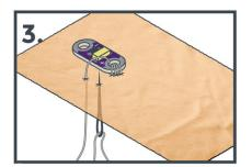
Pull the slack of the thread through so it sits flush with the fabric.
