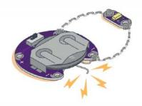
▲ One of the most common short circuits in e-sewing happens when a loose thread tail near the negative tab on the battery holder touches the battery. Always check your stitching before powering your project.
