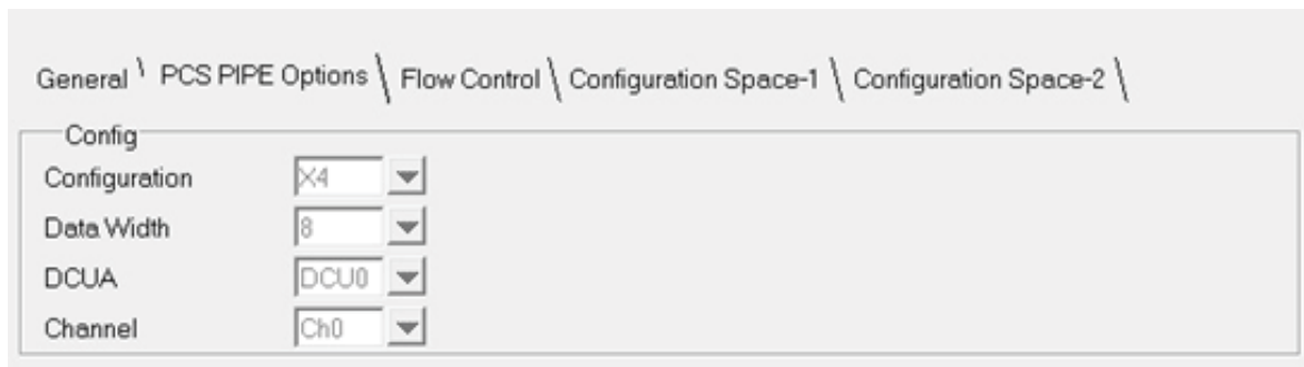
Figure 3.2. PCI Express IP Core PCS Pipe Options
