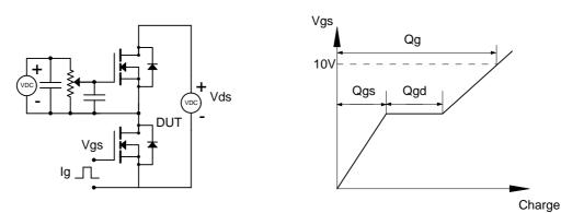
Resistive Switching Test Circuit & Waveforms
