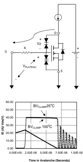
Fig 16: Unclamped Inductive Switching
